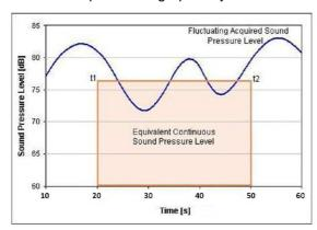
In EN 50332-1 the measurement time interval (t2 -t1) is 30 s.
